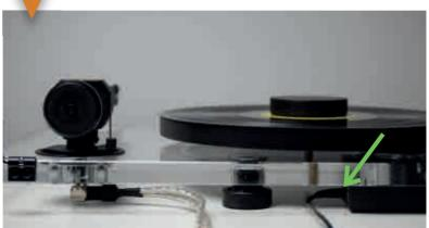
Use the rocker-switch on the left to select the playback speed.
