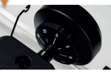
Turn the whole counterweight counterclockwise until the scale reads 18 - 20.
