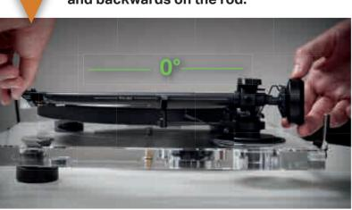
Turn the front dial of the counterweight (not the whole weight) so the '0' is in line with marker at the back of the tonearm.
